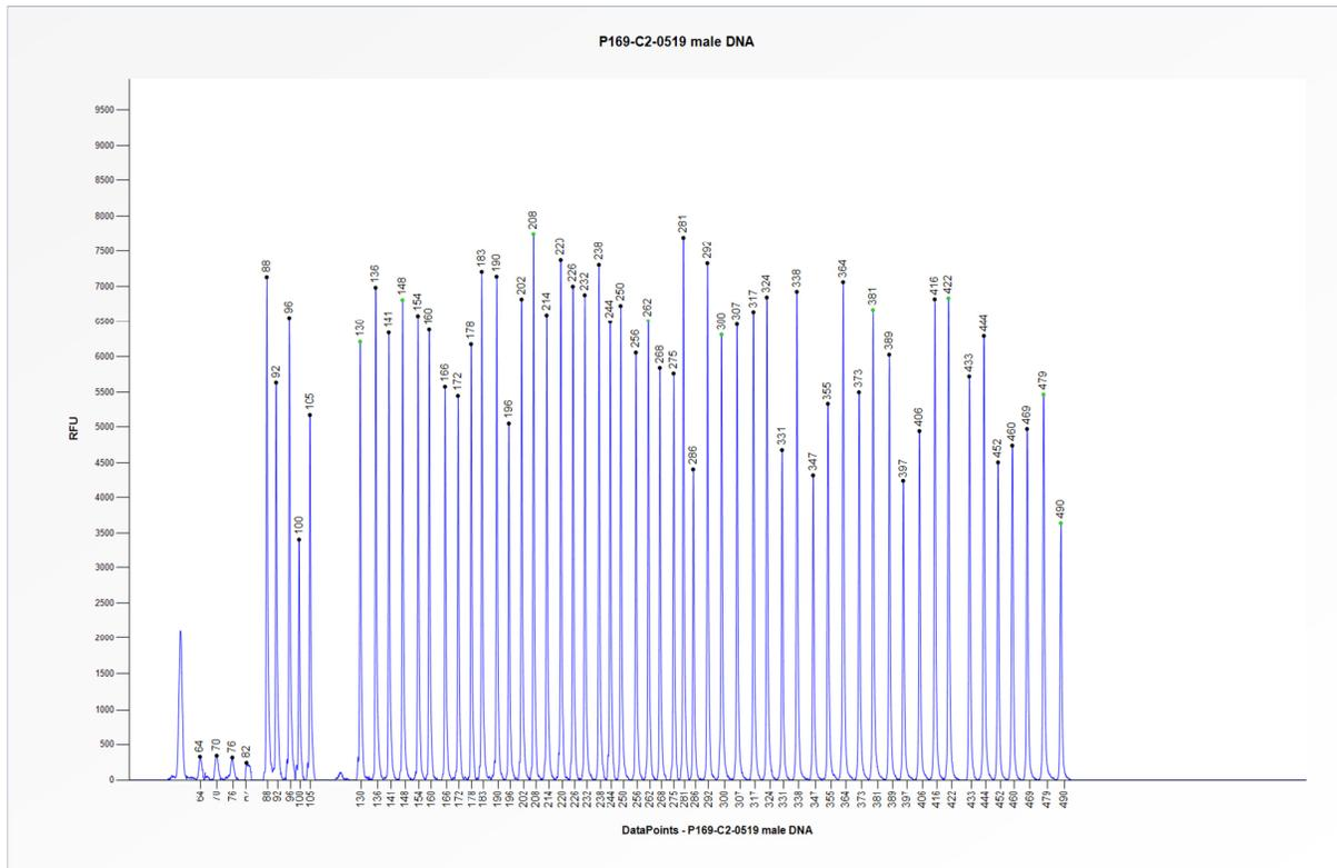
**Figure 1.** Capillary electrophoresis pattern from a sample of approximately 50 ng human male control DNA analysed with SALSA MLPA Probemix P169 Hirschsprung-1 (C2-0519).
